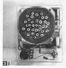
View showing holes drilled for speaker sound.
