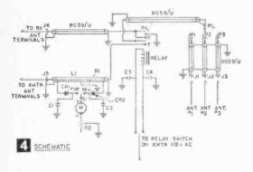
out a similar hole punched in the other end of the shield. Insert the insulated center conductor and spread the shield tight again. Wrap the shield ends with bare wire and solder to hold it in place. At midpoint from where the hookup wire enters and leaves the coax, spread the shield and pull a couple of inches of hookup wire out for connection of R1
