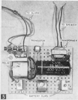
For easy assembly, use a perforated circuit board. Make the clips of scrap sheet metal.
