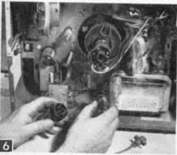
With cheater cord pulled out, the repairman carefully replaces an old tube with a new one. He works with one hand only to avoid shock.
