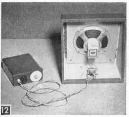
Optional speaker requires output transformer for correct impedance match to the 3.2-ohm voice coil.
