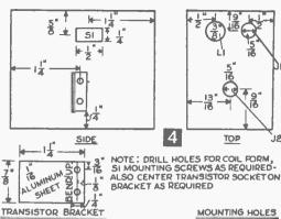
4, mount the coil form (with L1 and L2), input and output jacks (J2 and J1) at one end of the box. Attach the 1/16-in. aluminum transistor socket mounting bracket and "on-off" switch (S1) at the bottom center. Mount B2 vertically next to the transistor and B1 will then fit snugly into the remaining space
