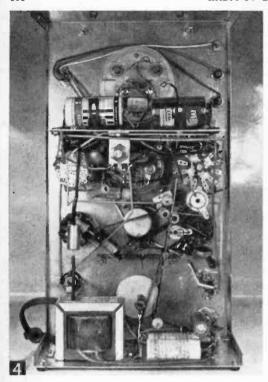
Interior view. Internal transistors are located on small chassis behind batteries.
