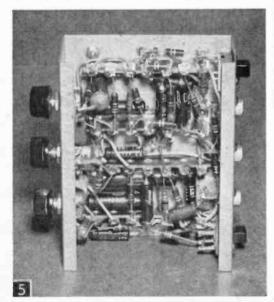
Completely wired chassis, bottom view.
