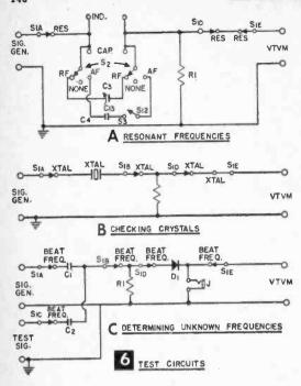
frequency. The amount of rise in voltage gives an indication as to the activity of the crystal. Its harmonic content can also be checked by tuning the signal generator to the crystal's harmonic frequencies.
