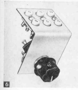
Three-channel crystal selector sub-assembly includes sockets, mounting frame and knob. Right, the three-point switch installed within a Knight-Kit T-50 amateur transmitter.
