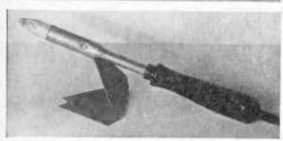
· You can stand or toss this temporary soldering iron rest onto the bench, and use it in whatever position it comes to rest. Shaped like
