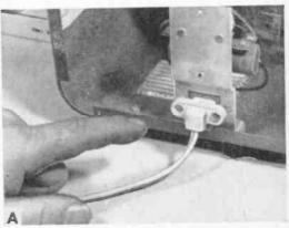
On this set, the cheater cord was originally riveted to the fiber back board. Rivets were removed so the cord could be used as a cheater.
