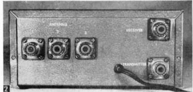
Coax jacks 1, 2, and 3 accommodate three different antennas. The two jacks on the right connect with coax cables from receiver and transmitter antenna terminals.
