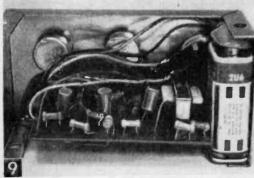
Amplifier completely assembled with battery tucked in place.
