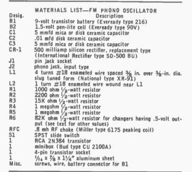
The audio voltage from the changer cartridge connected at J2 raises and lowers the bias voltage so that the diode shunt capacity change is proportional to the audio signal. CR-1 is connected in series with C3 across the oscillator coil so that the oscillator frequency changes with modulation. R5, like R4, is an isolating resistor.
