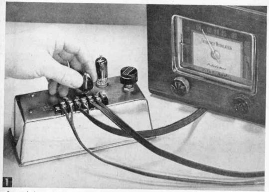
Connect the booster chassis to your FM tuner with a short length of twin lead. The other twin lead feeds out to the antenna.
