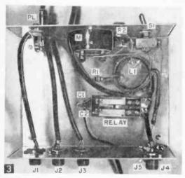
Cabinet is small, yet adequate for easy installation of components. Note short, direct two-conductor wire leads between phone jacks on front panel (top left) and coaxial jacks on back panel.
