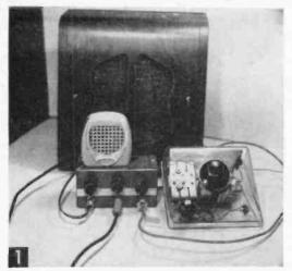
Amplifier connected to 6-in. speaker in baffle (output) and transistorized tuner (input).
