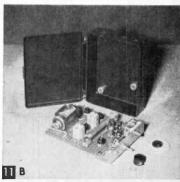
Two spacers cut from pipe are cemented to back of case to hold board in proper position.
