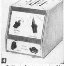
On the seconds range, you get a click every 1, 5, 10, 30, or 60 seconds. Each range has its own control pot on the back of the chassis for calibration.
