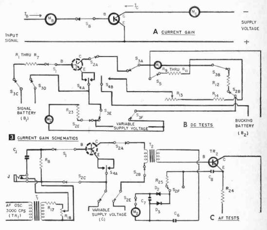
also reverses polarity, so that both PNP and NPN transistors can be tested.
