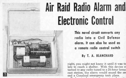
The complete circuit fits in a 4-in.-long plastic box. A single hearing aid battery provides 221/2-volt power.
