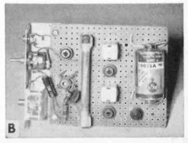
For a good wiring job, keep capacitors and resistors close to board and use spaghetti tubing an leads crossing bare leads or terminals to avaid shorts. Right, transistors shown in sockets on top of board where wiring is limited.
