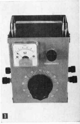
The campact impedance bridge simplifies antenna design and construction.
