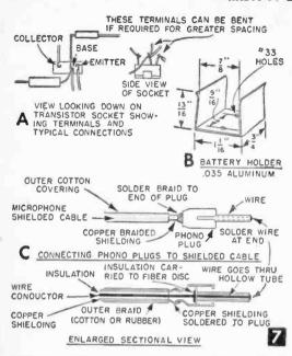
MATERIALS LIST-TRANSISTORIZED HI-FI PREAMPLIFIER No. Regd. Description 3 transistor sockets MS-275 3 G.E. 2N190 transistors 9 volt Burgess 2U6 battery male and 1 female battery snap-on clip or snap-on, two-terminal insert O.P.D.T. slide switch (SW17) D.P.S.T. slide switch (SW16) RCA type phono jacks and plugs 1 10-K ohm volume control with switch (K = 1000), miniature type VC-28
