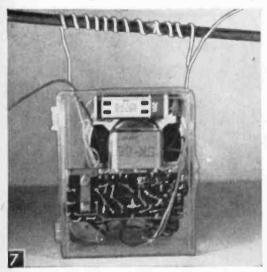
Rear view of crystal diode tuner encased with "Quickie."
