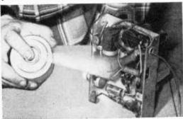
haves or goes dead. The trouble may be a part that expands with heat after current has been flowing through for a few moments. Spray suspicious parts with CO<sub>2</sub> gas one at a time. The intense cold will contract a defective component so it can work normally.
