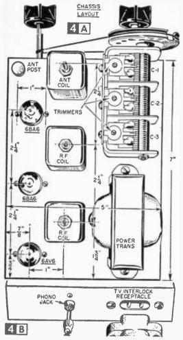
Your capacitor may be designed for horizontal operation. There is ample room on the chassis for either mounting.
