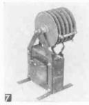
Alternate construction a full wave selenium rectifier mounted over the transformer. Both items can often be obtained in surplus stores.
