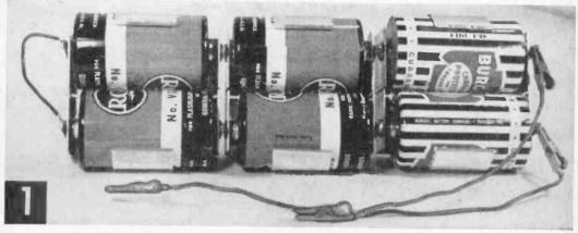
Complete power supply for transistor circuits and electrical experiments delivers 9 volts.
