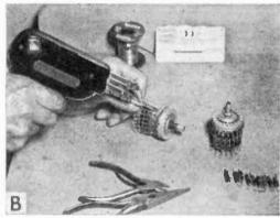
Shape resistor leads around two mails driven in a block of wood to get them of uniform length and with uniform loops (A); then, starting with terminal #1 on each switch with the lowest value resistor, position looped ends of resistors and solder at each terminal (B).
