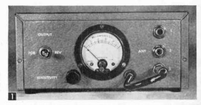
This convenient unit selects antennas, measures efficiency, and switches the antenna from receiver to transmitter.
