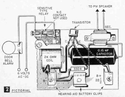
a sensitivity adjustment, advancing it to a level that provides the most satisfactory pickup and dropout of relay contacts. When properly adjusted, the circuit should not be affected by music or speech, but only by the absence of the station's inaudible carrier, which will cause the alarm to draw current and close the relay alarm contacts.
