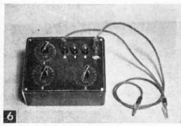
Completed job shows the lettering that was put on with decals sold for the purpose. After decals have thoroughly dried, apply a thin coat of clear plastic with a small brush to make them permanent. Banana plugs and clips soldered to short flexible leads make connections quick and easy.
