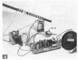
Tuner cambined with powerful sub-miniature, fivetransistor amplifier. All companents can be attached to the breadboard or installed in an ald radia cabinet.
