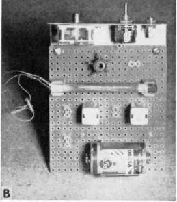
Left, underside of board showing socket and IF transformer terminals prior to wiring. Right, major components mounted on top of board. Spring clip holds battery; fuse clips the antenna coil.
