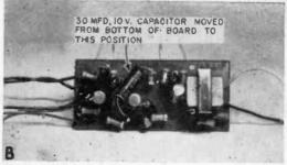
Modifying the amplifier with a resistor added on under side of printed circuit board (left) and a capacitor moved to top side (right).
