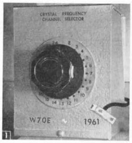
External 24-channel crystal frequency selector fitted with coaxial cord and plug to fit crystal socket in the transmitter.
