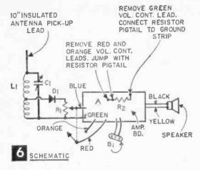
Now position the amplifier for mounting. Pass the two pieces of solid wire through the inside of the speaker magnet frame, bend them around the outside of the frame, cut them to length, and solder them to the ground
