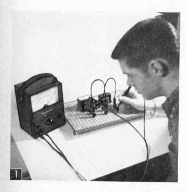
Simple 11-step power supply offers a variety of voltages to operate tube heaters, test intermittent equipment, correct line current and handle other applications
