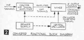
cost. Use of a command receiver with the VHF converter has the advantage of providing a completely independent VHF receiving installation, so that other receiver equipment remains free for normal use.
