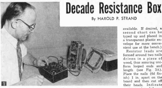
Decade resistance box in use in radio servicing job. Various values of resistance are being applied across terminals where a defective resistor was formerly soldered, and which is now unidentifiable due to extreme heating.
