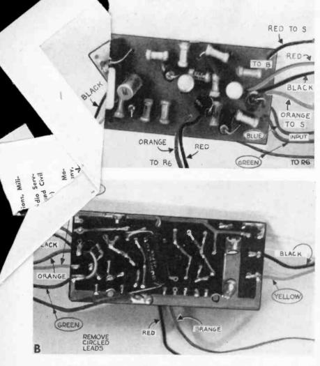
Top view of printed circuit amplifier showing colored leads. Be sure to read instructions packed with this board.
