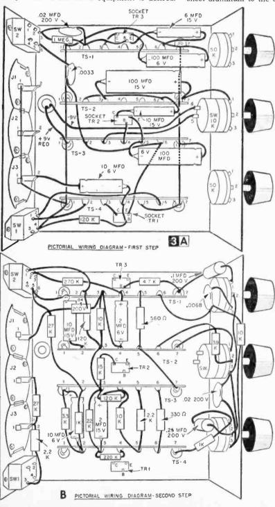
strip, one in a drilled hole %16 in. away — and press the rubber grommet in its hole. Cut off the shafts on all three controls to about ½ in. before installing them unless the extra length of shaft is required for mounting in a cabinet.
