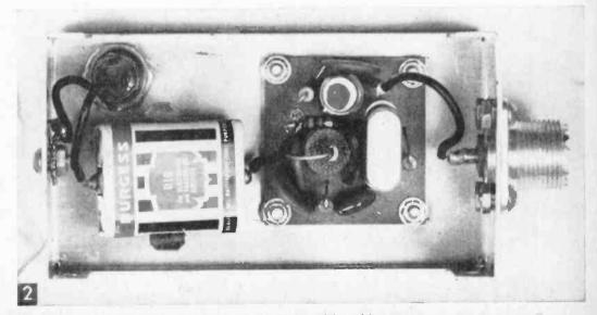
Underview shows printed circuit module and battery.
