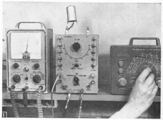
Determining resonant frequency of coil-condenser combination with VTVM at left and signal generator at right. Coil-condenser combinations may be connected to either set of terminals.
