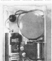
Top view showing high-pressure pushbutton switch.
