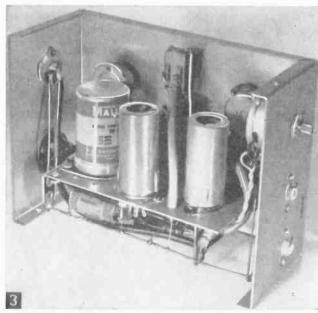
Back of panel view of mixer with cover removed. Note Input jacks and Hum Control on end panel at right.
