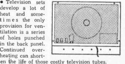
To get more ventilation, replace the panel with a simple frame covered with plastic screen such as is shown above.-W. H. McClay.
