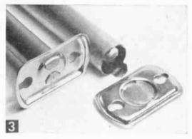
Remove tube flange by prying lugs out with a screwdriver. Do not cut or bend lugs back until pole has been installed in base.
