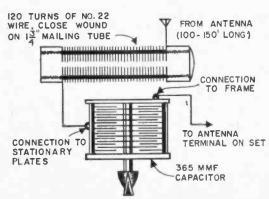
7 OPTIONAL ANTENNA TUNING SYSTEM FOR DX
