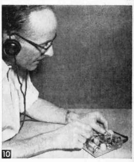
Listening in on an antenna trimmer adjustment, and af several steps in aligning the set.
