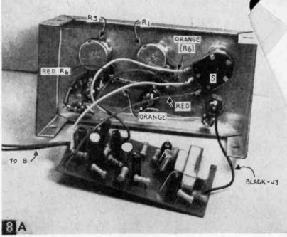
Connecting the printed circuit board to the switch and jacks.
