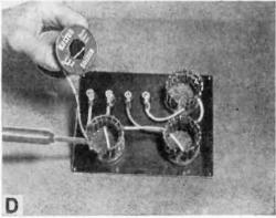
With the resistor-equipped switches attached to the panel, attach tormed rings of bare copper wire to free loops, bending them down uniformly over the ring (C); and after the three rings have been placed and leads connected as shown, solder all points of contact to the rings (D).
