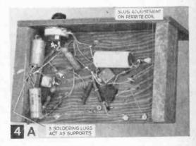
Underside of chassis shelf offers plenty of wiring room. Insulated staple on left shelf support protects line cord from undue strain.
