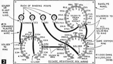
solder (Fig. 3B). As shown in Fig. 2, the #1 terminal is at the right side of the wide spacing on the switch contacts.
