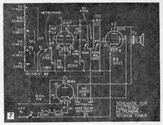
Calibration is Next, after a wiring check. Turn S3 to "seconds" and S2 to the one-second position. Turn the unit on with volume about half way up. You should hear ticks from the speaker in about 30 seconds. Allow a ten minute warm up period, and then use an electric clock second hand to adjust pot P1 until the click frequency is exactly one per second. Pot P1 is left in this position throughout the rest of the calibration.
