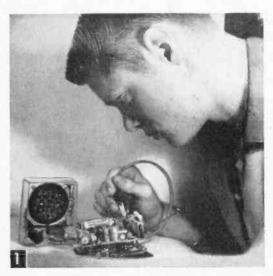
Tracing a signal in transistor radio.
