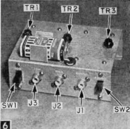
The designations TR1, TR2 and TR3 indicate the transistors; SW1 is the low or high level switch; J3 is the low impedance input; J2, the high; J1, the output; and SW2 is the phono or mike switch.
