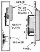
THE METER IS HELD IN PLACE ON THE PANEL BY THE METER CLAMP BRACKET
