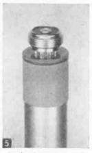
Insulated installation of connector, ready for any standard mike.
